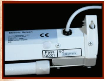
This is the power end of the case. The power cable connection looks different than yours but the location and function of the limit switches will remain the same. You can see a rubber plug just above the word Pass on the casing.
