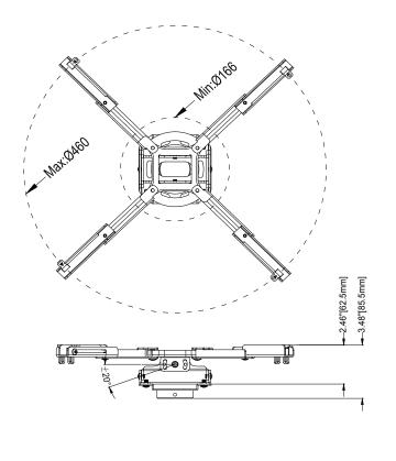
Heavy duty all steel construction in a very low profile package. Multiple (12) adjustment points for extra grip with heavier or off-center of gravity projectors. Comes completely pre-assembled for a quick installation and features a quick release for bulb replacement.
