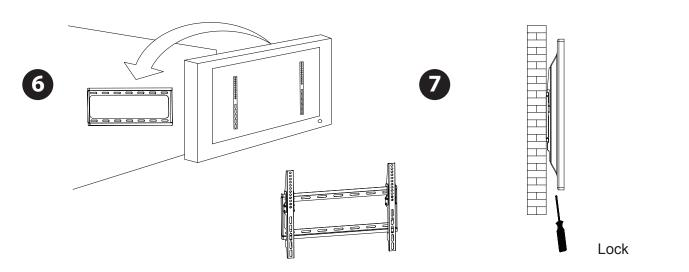
Tighten or loosen the screw to make the tilt happen.
